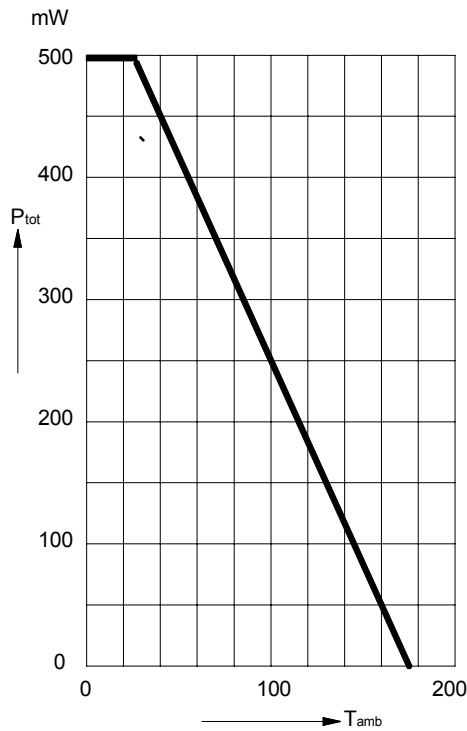
FIG.2 – ADMISSIBLE POWER DISSIPATION VERSUS AMBIENT TEMPERATURE
